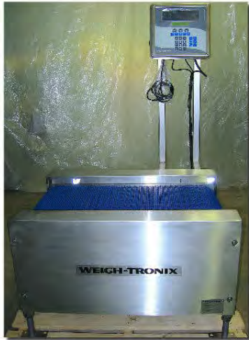
Custom Stand and Indicator Mount for Weigh Tronix Scale Accompanying Product Reject Mechanism
