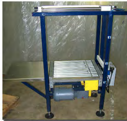
Custom Stand and Indicator Mount for Weigh Tronix Scale Accompanying Product Reject Mechanism
