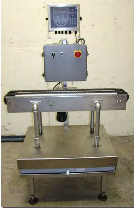
Two Strand Chain Conveyor Barcode validation application Caustic/Corrosive Environment Remove-able Conveyor
