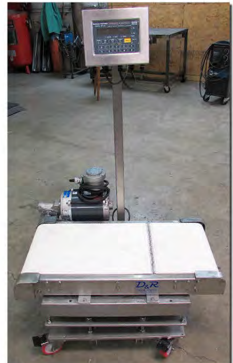
Rough Top Belt Conveyor Bagging Application Nema 7 XP Controls
