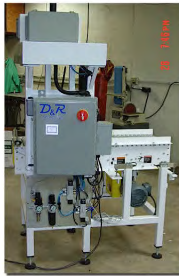
Live Roller Conveyor Pop-Up Product Stop Over / Under Reject Leveling Feet
